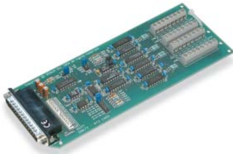
The 8-channel DBK9 RTD card accommodates 3- and 4-wire RTDs
